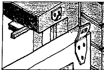
4. Hook to suspend the storm-window: It is advisable to install weather stripping on the frame or caulking on a seasonal basis.
